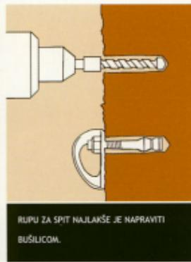
RUPU ZA SPIT NAIKLJEŠE JE NAPRAVITI BUŠILICOM.
